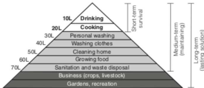
Figure 9.1. Hierarchy of water requirements (after Maslow’s hierarchy of needs)
