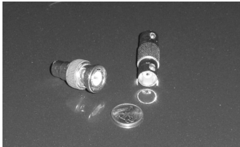
Male (left) and female (right) BNC connectors
