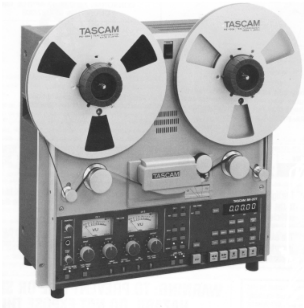
Tascam BR-20 Reel-to-Reel Recorder often used in SA community radio stations
