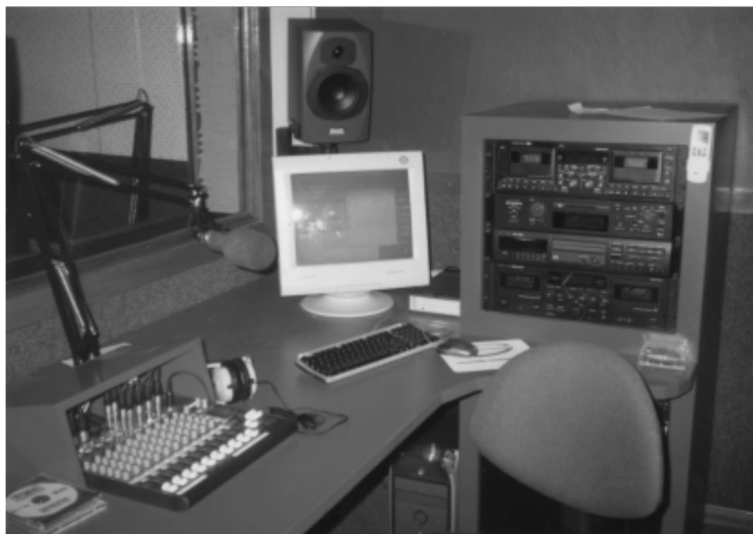
Production studio at Radio Graaff Reinet, in the Eastern Cape. The mixer, digital editing system and equipment racks can be clearly seen.
