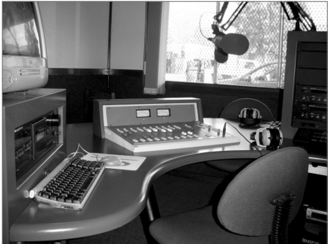
Broadcast studio at Radio Graaff Reinet. The broadcast mixing desk, presenter's microphone and playout computer can be clearly seen.
